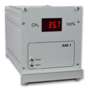
The gas analyzer GAE is a non-dispersive infrared-photometer (NDIR). It records the absorption of infrared rays, caused by the measuring gas. The wavelengths of the absorption bands characterize the type of gas, whilst the intensity of the absorption is a measurement for the concentration of the measuring components.
